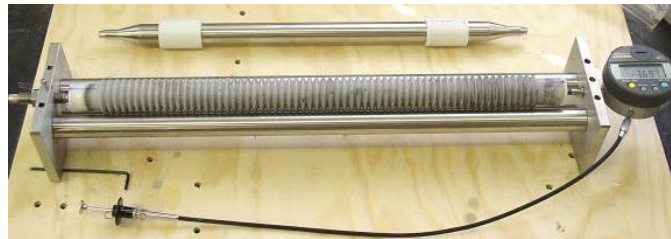
Figure 3.11. Autogenous shrinkage specimen in dilatometer.
