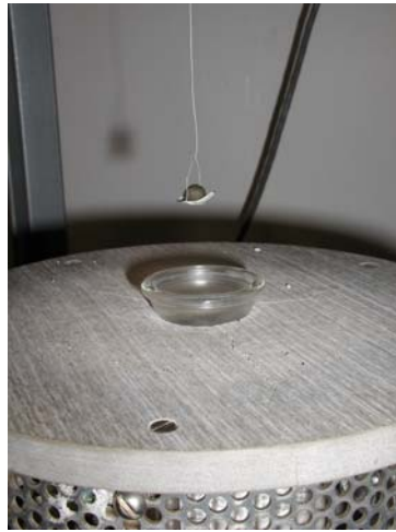
Figure 3.9. TGA specimen in titanium boat.
