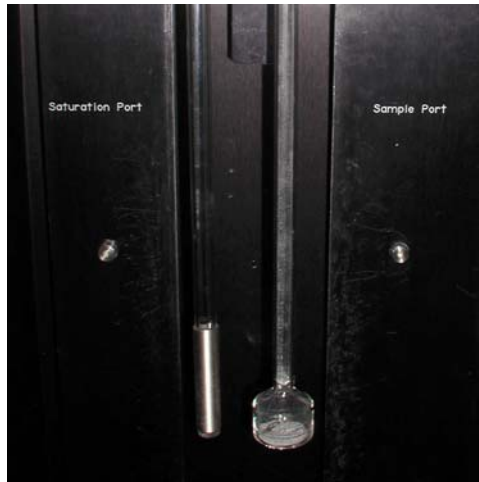
Figure 3.12. Sample flask used for BET and BJH testing.
