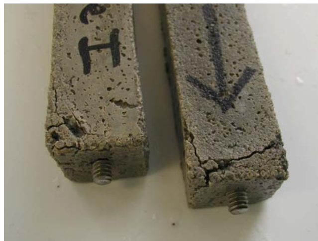
Figure 4.33. Image of 8% MK235 mortar prisms after 300 days of sodium sulfate exposure.
