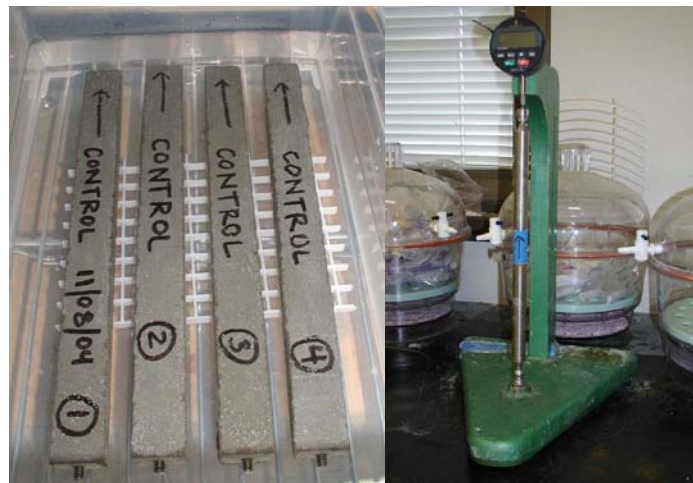
Figure 3.17. Mortar prisms (left) and electronic comparator (right).
