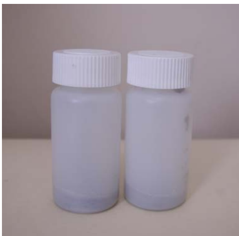
Figure 3.7 Polyethylene ampules used for isothermal calorimetry.
