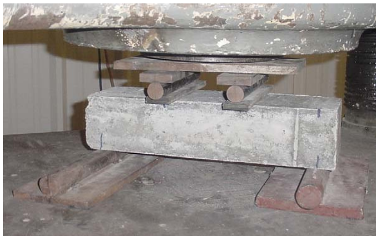
Figure 3.14. Third-point loading experimental configuration.
