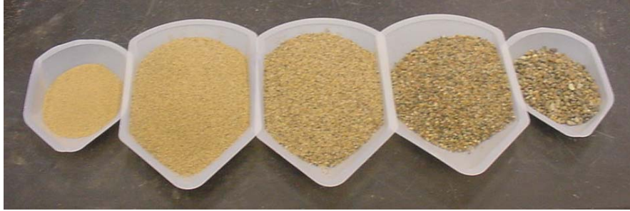
Figure 3.5. Alkali-reactive sand used in ASR test, ASTM C 1260.
