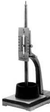
Figure 3.6. Vicat needle apparatus [Humboldt Manufacturing - Vicat Consistency Testers].
