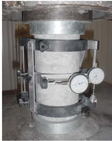
Figure 3.15. Method for determining modulus of elasticity in compression.
