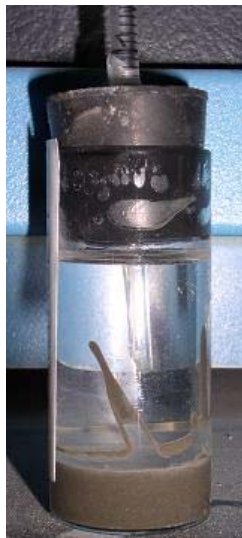
Figure 3.10. Chemical shrinkage setup.
